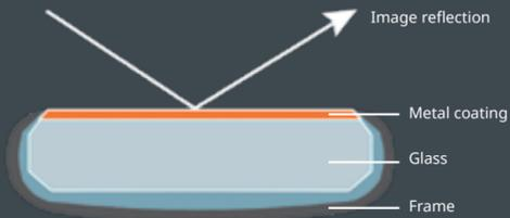
Image reflected directly on the surface of the glass, distortion-free
